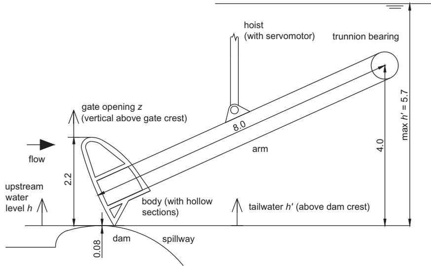
Figure 1. Definition sketch of a prototype radial gate above a curved dam. Dimensions in metres.
