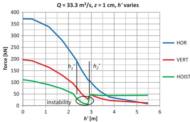
Figure 8. The effect of  $h'$  on forces for constant  $Q$  and  $z$ .
