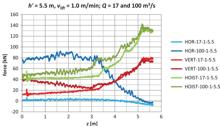
Figure 3. Forces during  $v_{\text{lift}} = 1.0$  m/min at  $h' = 5.5$  m for  $Q = 17$  and  $100$  m<sup>3</sup>/s. Denotations in the legend: force (HOR, VERT, HOIST) [kN]– $Q$  [m<sup>3</sup>/s]– $v_{\text{lift}}$  [m]– $h'$  [m].
