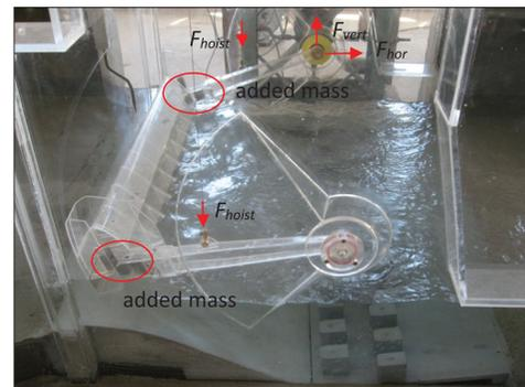
Figure 2. Side view of the 1:17 scale model with positive directions of measured forces.
