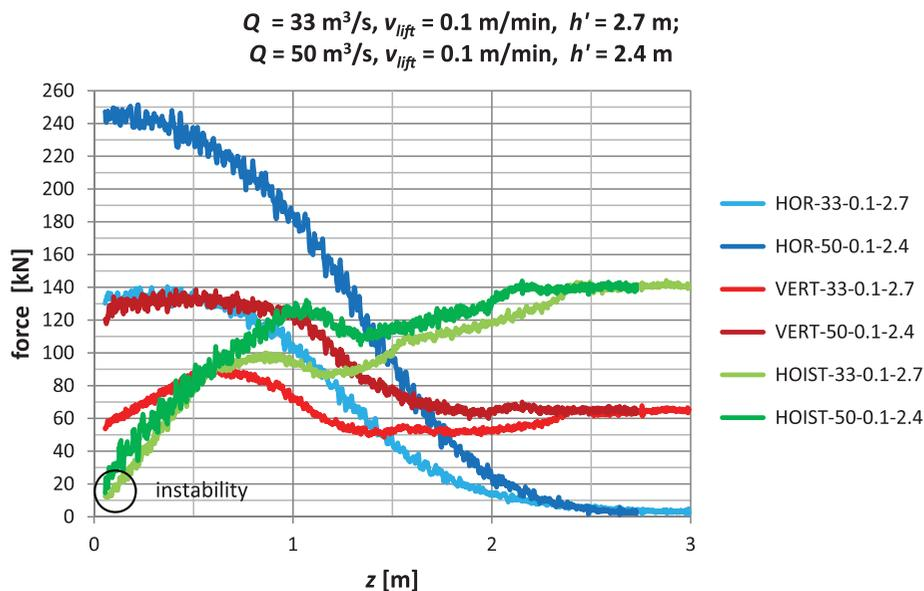
Figure 5. Examples of initially unstable gate becoming more stable during the lift. Denotations in the legend: force (HOR, VERT, HOIST) [kN]– $Q$  [m<sup>3</sup>/s]– $v_{\text{lift}}$  [m/min]– $h'$  [m].
