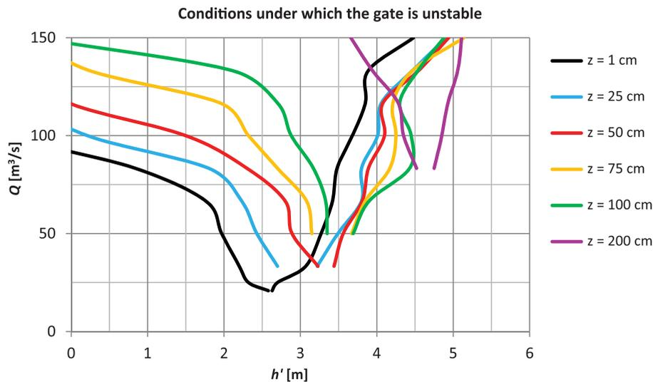
Figure 9. Combinations of  $Q$ ,  $h'$  and  $z$  when the gate was unstable. Equally coloured pairs of lines, denoted  $z = \text{const.}$ , represent values  $h'_1$  (to the left) and  $h'_2$  (to the right side of diagram) for a given  $Q$  and  $z$ .
