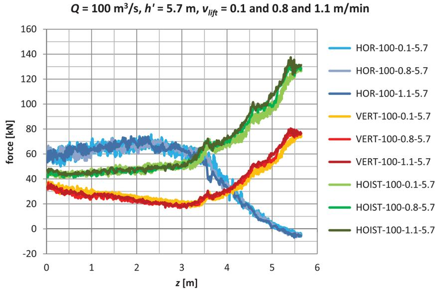
Figure 4. Forces at  $Q = 100 \text{ m}^3/\text{s}$  and  $h' = 5.7 \text{ m}$  for  $v_{\text{lift}} = 0.1$  and  $0.8$  and  $1.1 \text{ m/min}$ . Denotations in the legend: force (HOR, VERT, HOIST) [kN]– $Q$  [m<sup>3</sup>/s]– $v_{\text{lift}}$  [m/min]– $h'$  [m].
